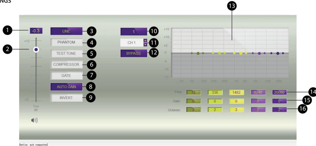
1. Input level value | 2. Input level fader | 3. Gain selector | 4. Phantom power switch | 5. Test tone generator | 6. Audio compressor | 7. Gate setting | 8. Auto gain | 9. Phase inverter | 10. Input name | 11. Input selector | 12. Bypass button | 13. Parameter equalizer | 14. Center frequency indicator | 15. Amplitude indicator | 16. Bandwidth indicator
